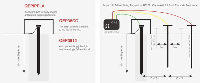
If the required resistance is not low enough additional rods are installed to make the depth greater until the resistance is lowered to the required value.
